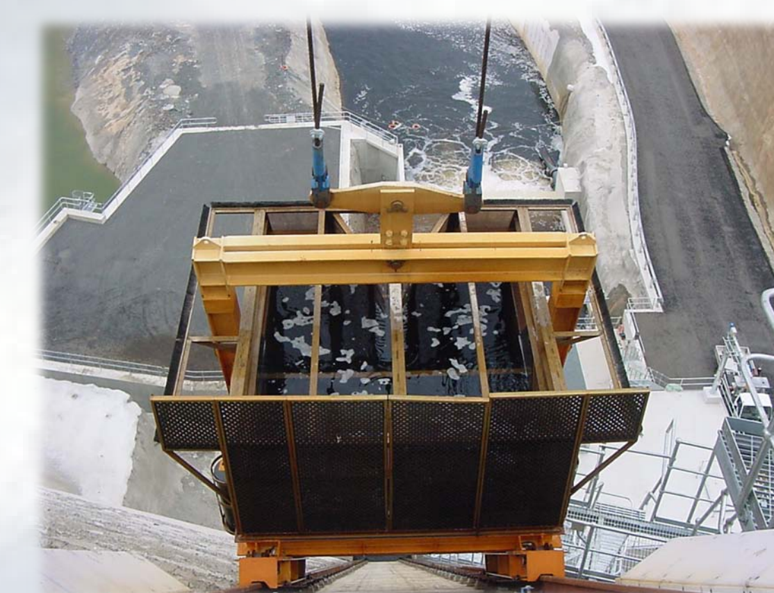
Fish Elevator in Australia, 10
