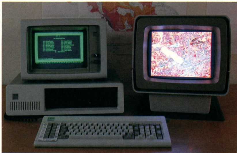
Figure 1. Basic Image Processing Workstation, IBM XT with a 670 × 480 Resolution, 9 Bits (512 Colors) Monitor.
