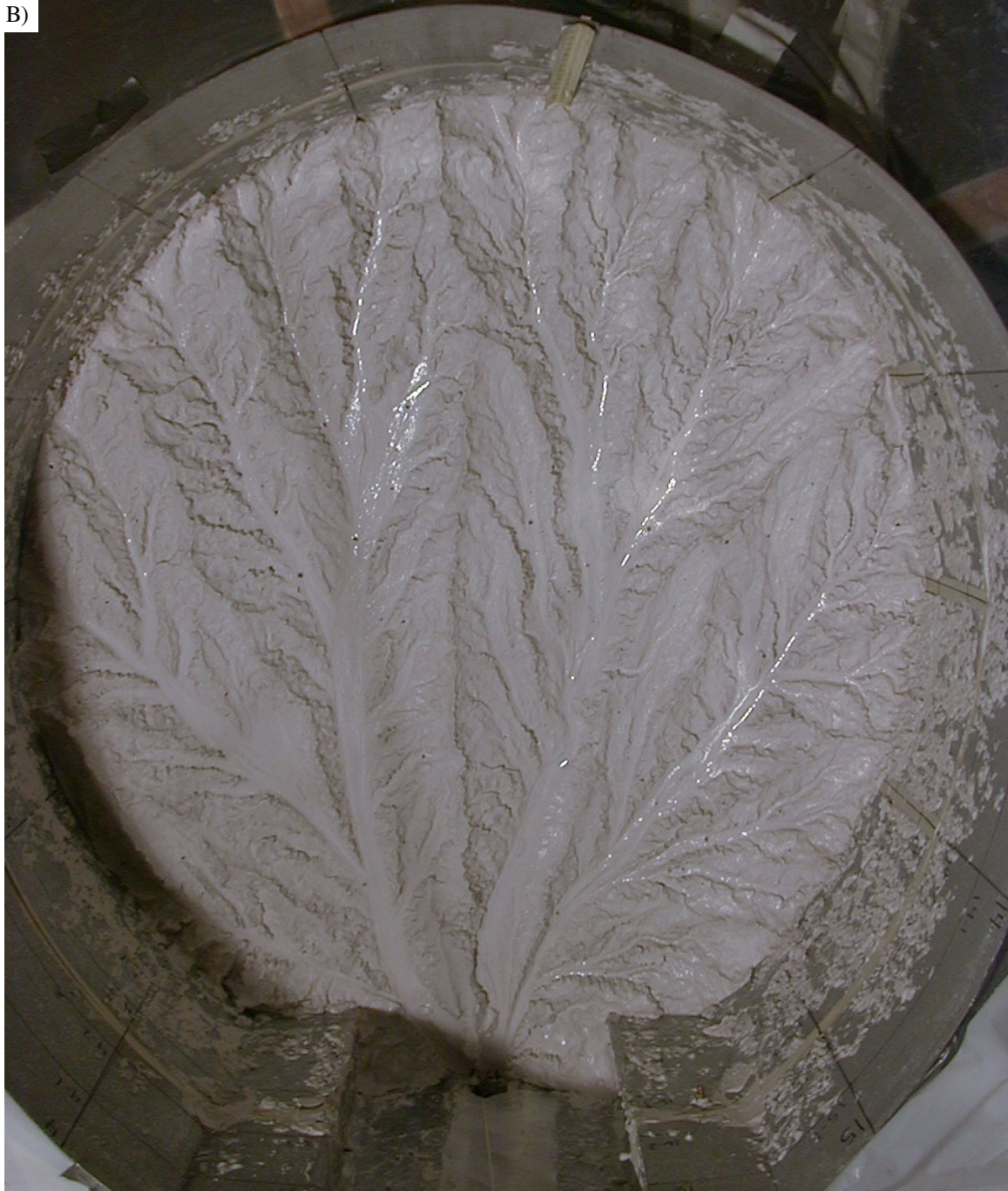
Figure 2-26. B) Surface after an additional 20 cm of erosion ( 1.2 H_r ), a long pause in base level fall, and subsequent initiation of steady run conditions (time = 395,000; Fig. 2-25). Maximum relief is 17.2 cm.
