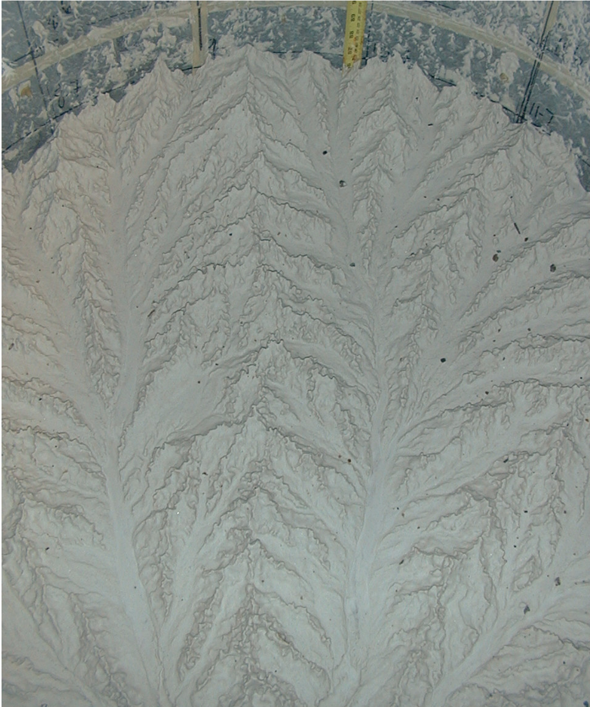
Figure 2-28. Oblique view of the surface at the end of run 5, demonstrating the crenulated, rough character of the ridges. Width of view is approximately 50 cm. A knickpoint is barely discernible in the bottom right center. This same knickpoint is seen more clearly in Fig. 2-27.
