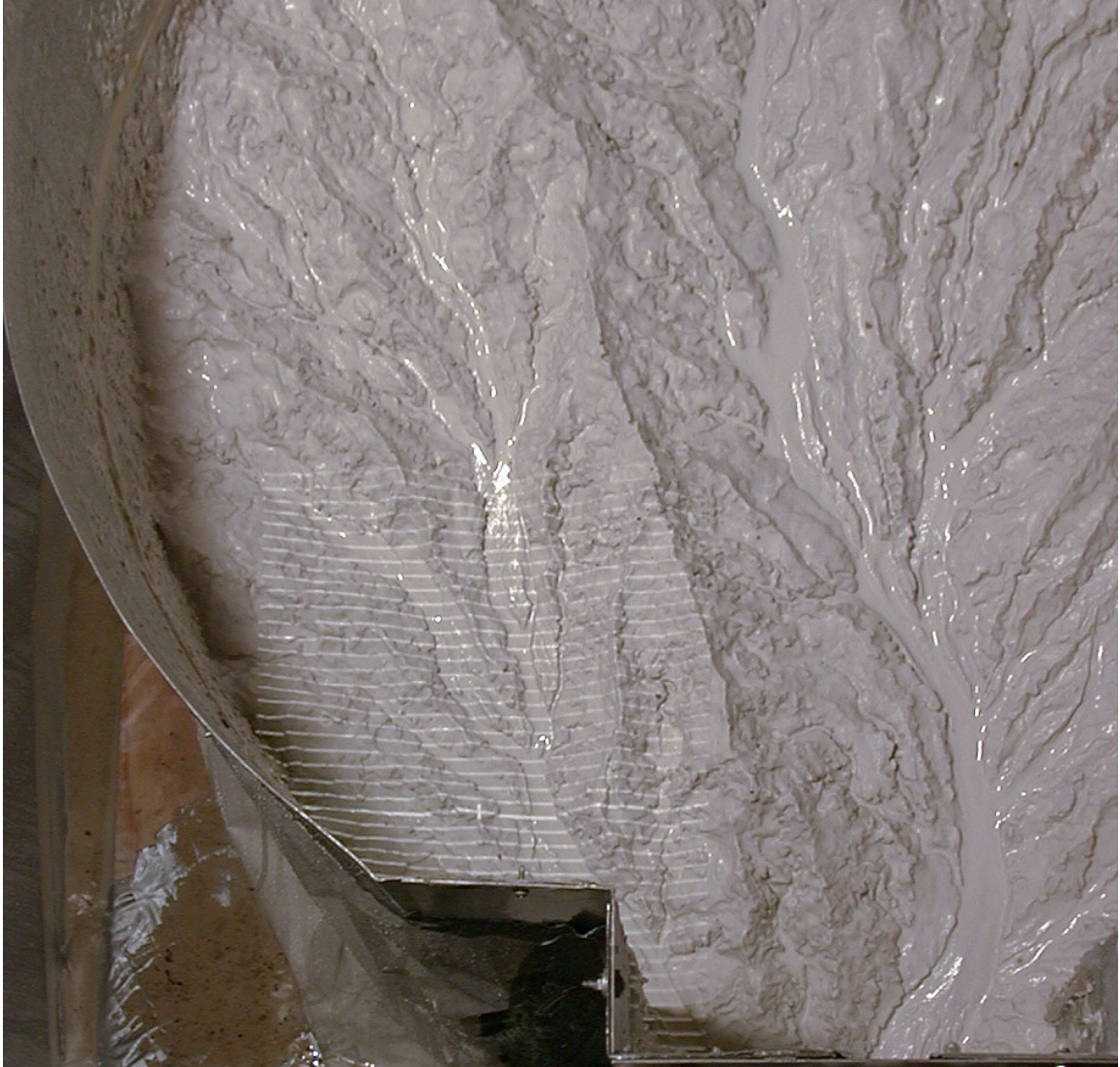
Figure 2-20. Sub-vertical view of surface after 18 cm of erosion since complete dissection ( 0.75 H_r ). Several hillslope failures are visible as scalloped sections along ridges. White lines in lower left are projected parallel lines from a slide projector above the tank. Width of image is ~50 cm. Terraces are visible along the lower right hand side trunk stream. The valley floors tend to be quite smooth, with poorly defined channels.
