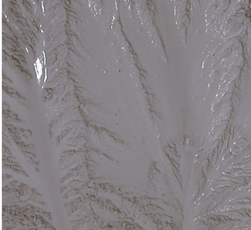
Figure 2-3. Sheet flow reduces relief and smooths the surface. Width of image is 17 cm. Note the knickpoint in the lower right.
