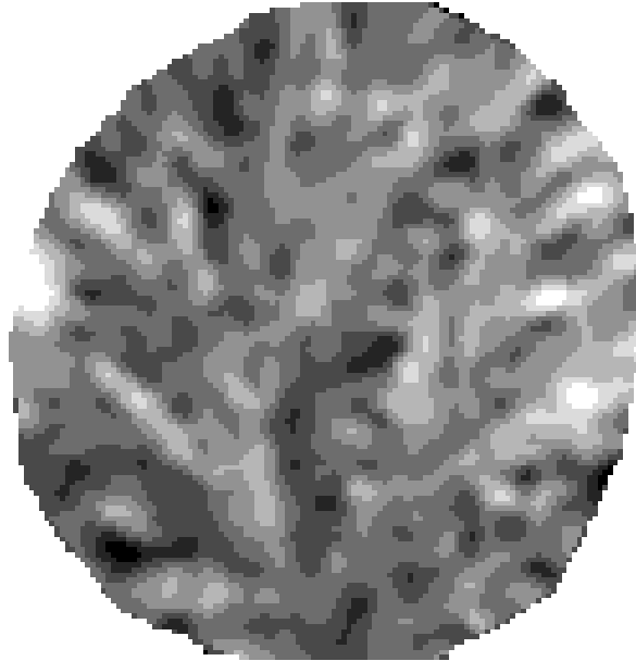
Figure 4-3. Spatial erosion rates plotted as a gray scale bitmap (8 grays), computed for grids from run 4 separated by 8 cm of erosion ( \sim 0.5 h/H_r ). White indicates high erosion rates, and dark indicates low erosion rates. Average erosion rate is 0.59 \mu\text{m/s} (long term average from base level curve is 0.55 \mu\text{m/s} ), with a one standard deviation ( \sigma ) of 0.19 \mu\text{m/s} ( \sigma/\mu \sim 0.33 ).
