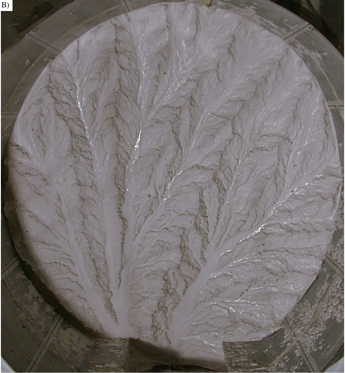
Figure 2-30. B) Surface after an additional 22 cm of erosion, run 6. Maximum relief is 14.3 cm.
