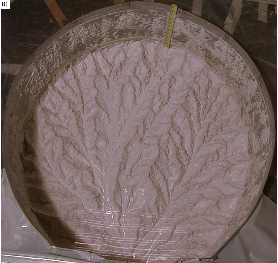
Figure 2-24. B) Surface after an additional 22 cm of erosion ( 1.3 H_r ).
