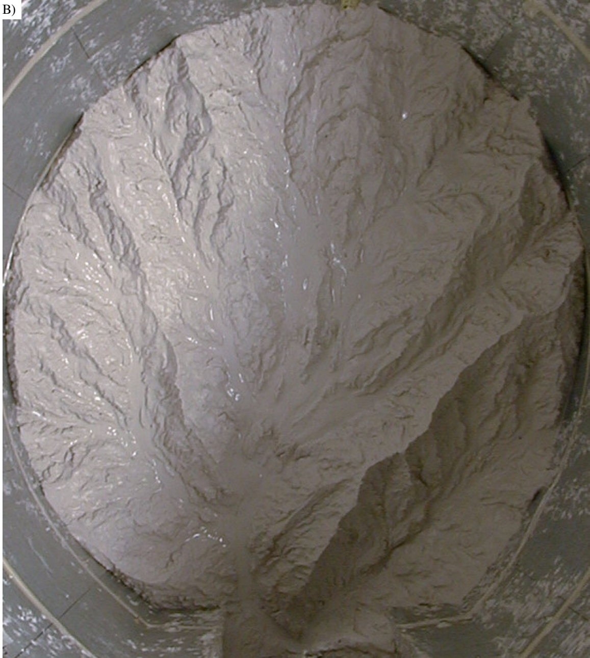
Figure 2-22. B) Surface after additional 1 relief unit of erosion. Two knickpoints are visible below center and another closer to the outlet. Scalloped ridge crests, indicative of hillslope failures, are visible along the longer ridge in the left of the photograph. Terraces are visible in the lower right hand drainage.
