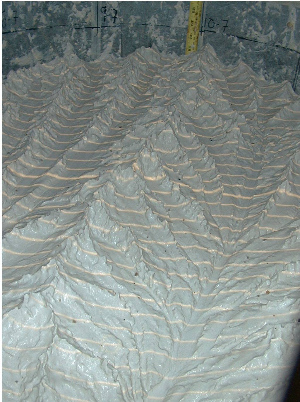
Figure 2-31. Close-up view of surface at steady forcing from rainfall and uplift, nearing the end of the run. Lines are projected from a slide projector. Width of view is approximately 40 cm. Surface is relatively smooth.
