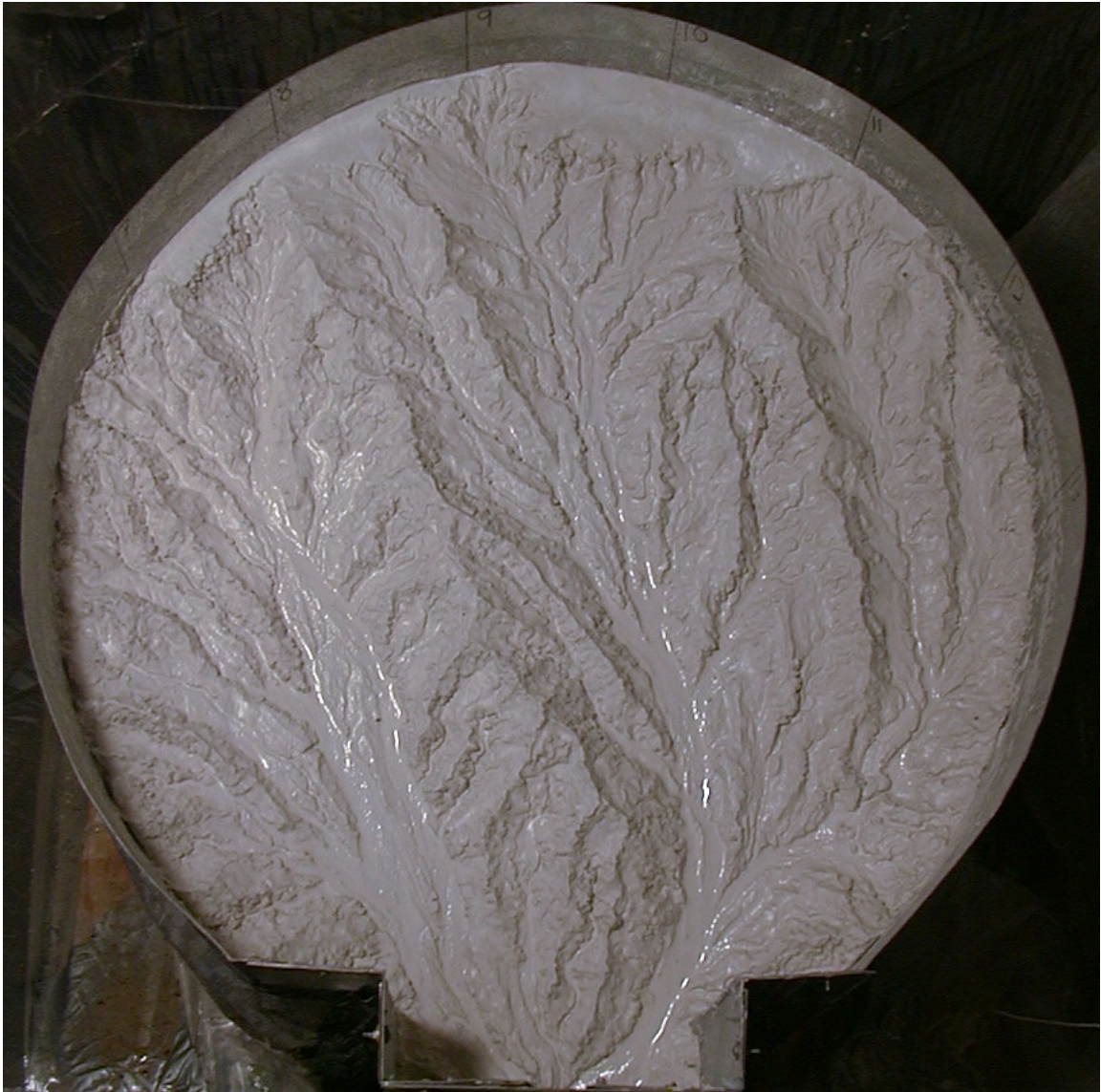
Figure A-2. Vertical photograph of drainage basin nearing complete dissection. Note that upper right corner retains remnants of initial flat surface. Basin is 87 cm wide, 98 cm long. Original digital photograph is 1280 × 960 pixels.
