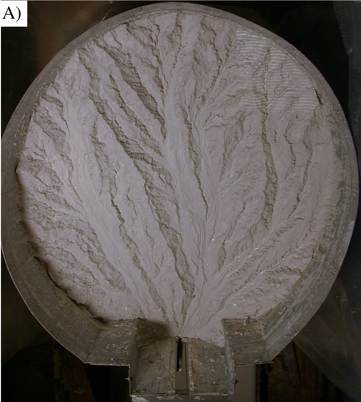
Figure 2-19. Vertical photographs of A) surface at complete dissection; and B) surface at the end of the run, after \sim 3 H_r of erosion. Basin width is 87 cm. Note the poor correspondence of ridge locations between the two images.
