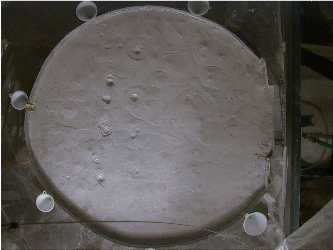
Figure 2-4. Initial surface condition prior to erosion. Outlet to basin is on the right. Smoothed mounds are remnant mud volcanoes. Holes are from persistent drips during rainfall calibration. An initial stream pattern has developed in a few places. Basin length (from left to right) is 99 cm.
