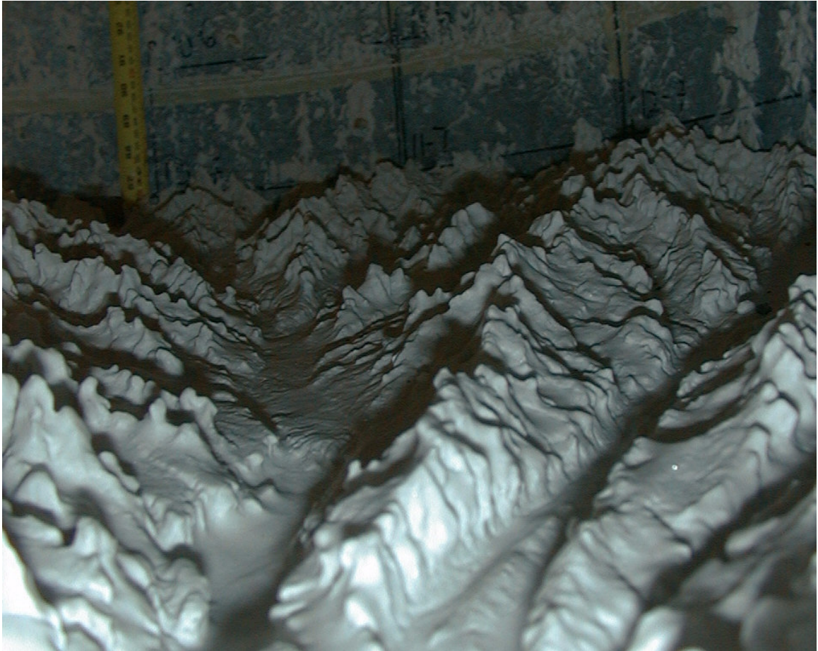
Figure 2-27. Low angle photograph of surface at the end of run 5. Width of image is approximately 30 cm. Note tape measure at top left. Numbers on left of tape are inches and on right of tape are cm. A knickpoint is visible in the main channel on the left side of the photograph. Terrace-like structures were left in the wake of the knickpoint. Note the ‘peaky’ nature of the ridges, and the smooth valley floors.
