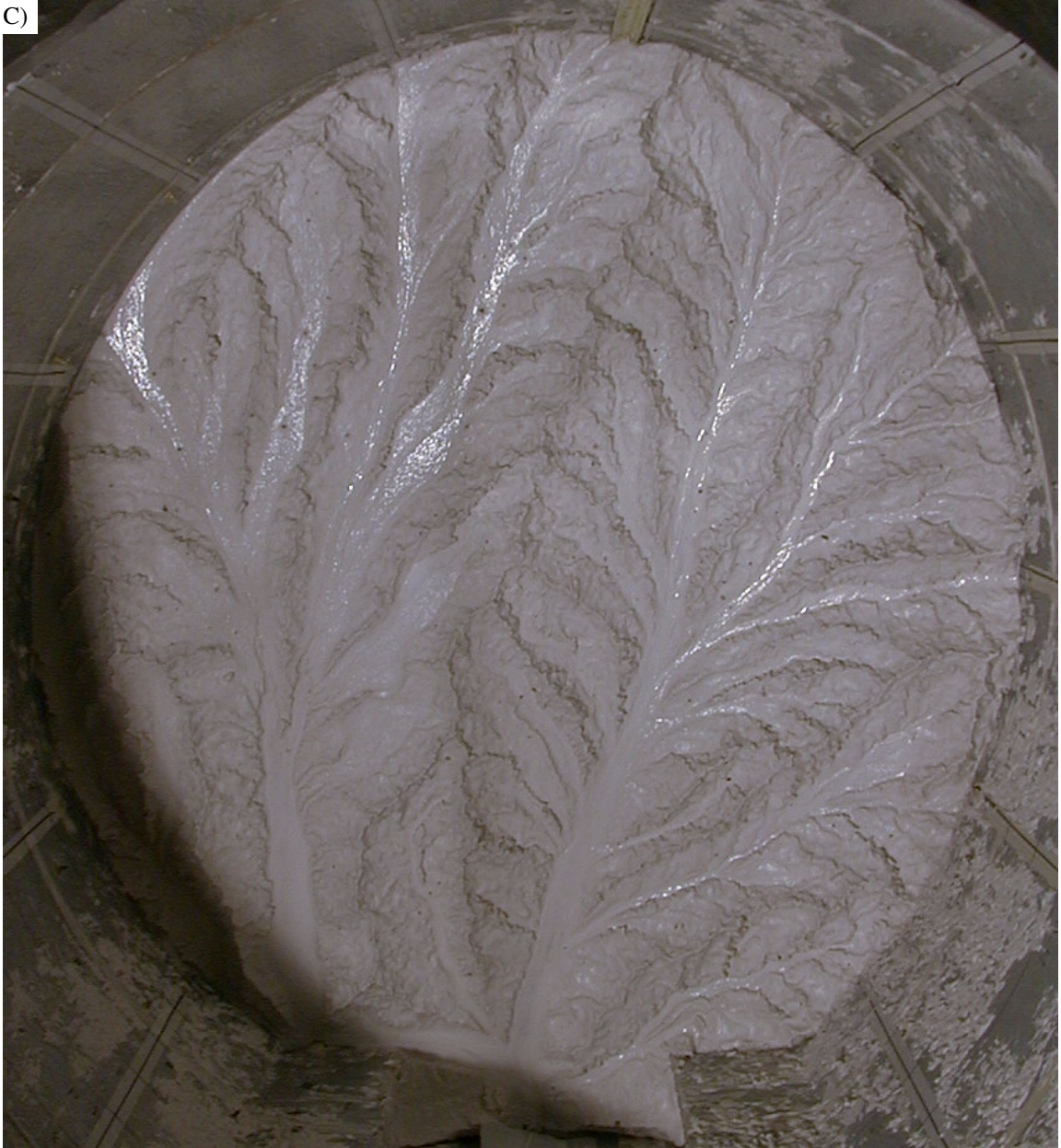
Figure 2-30. C) Surface at the end of the steady forcing portion of run 6. Maximum relief is 16.8 cm.
