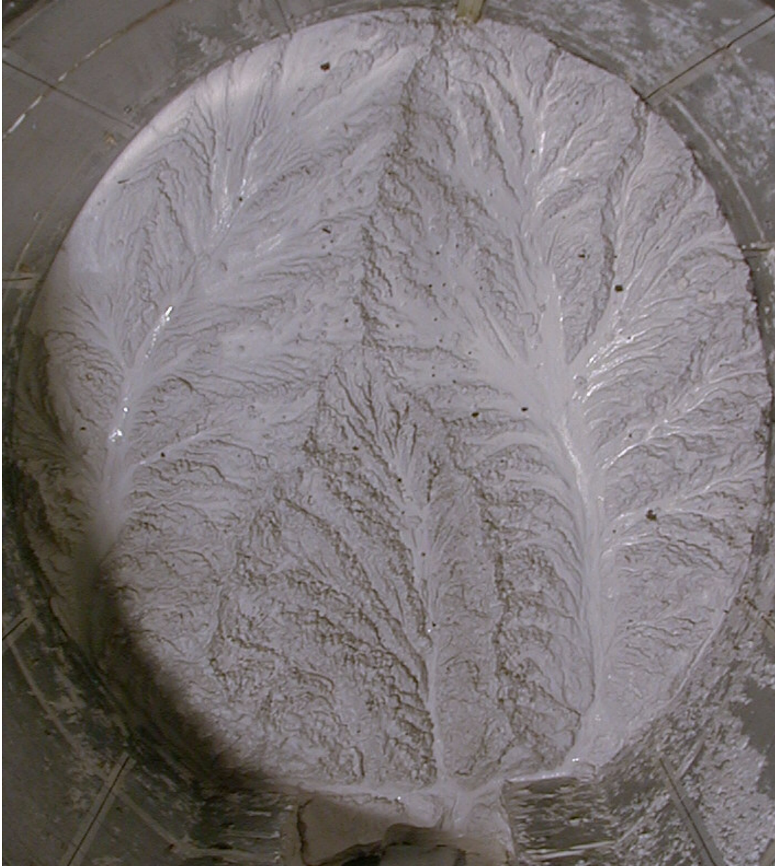
Figure 2-38. Surface just prior to cessation of base level fall, run 7. Width of basin is 87 cm. Lower center portion of basin has roughened considerably as a new sub-basin has grown upstream from the outlet. The two large trunk streams have migrated toward the edges of the basin. Smoothest regions of topography also mark the locations with the highest rainfall rates.
