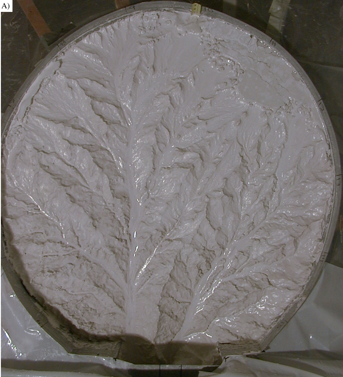
Figure 2-24. A) Surface nearing complete dissection, run 4. Hillslopes appear rather smooth, with concave hollows at valley heads. Width of the basin is 87 cm.
