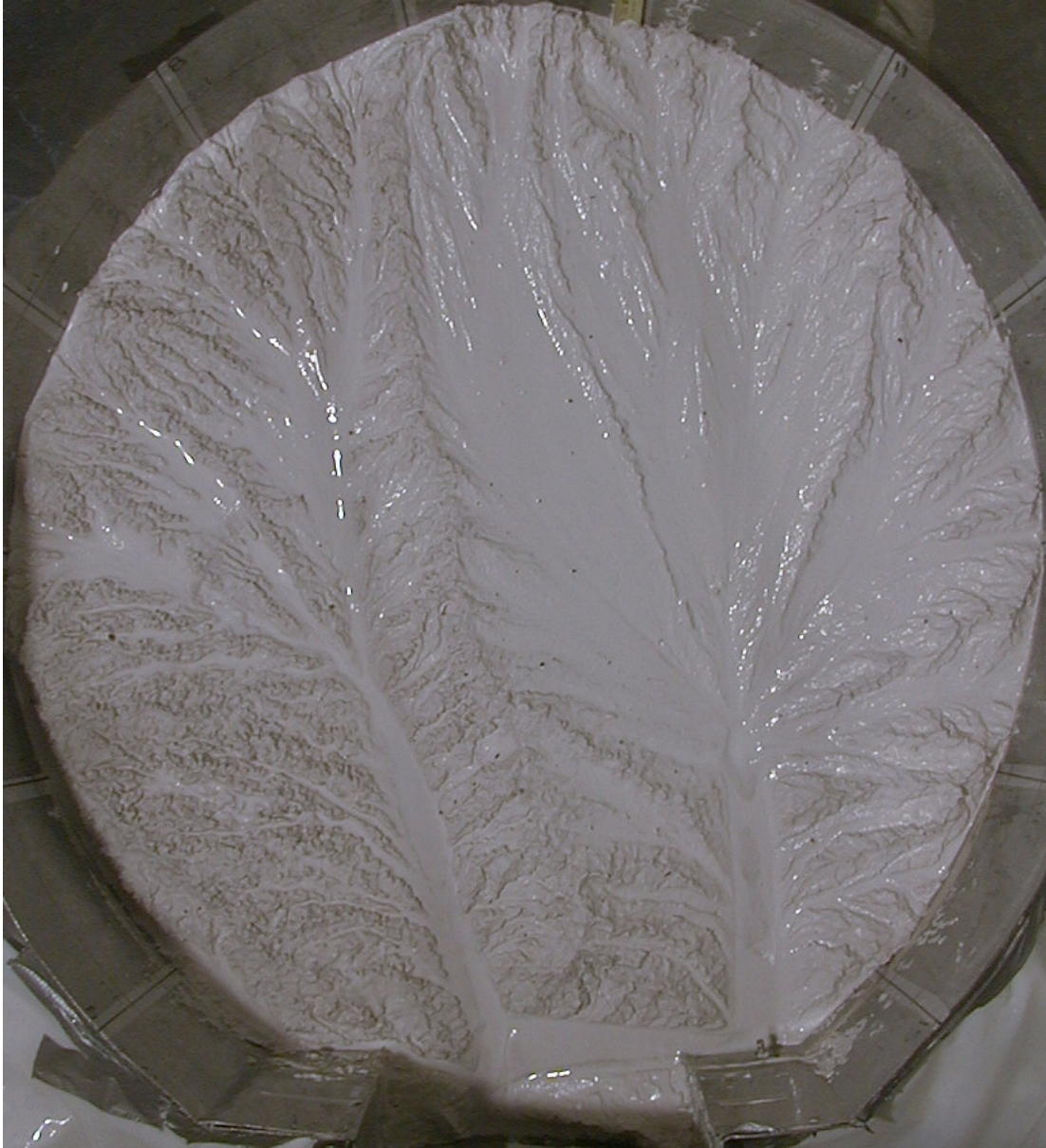
Figure 2-36. Surface just prior to the mist apparatus adjustment at t = 66,000 s, run 7. Note the smooth character of the right side sub-basin. A scour hole is visible in the right side trunk stream where flow converges from several sub-basins. In general, the roughest regions correspond to the lowest rainfall rates.
