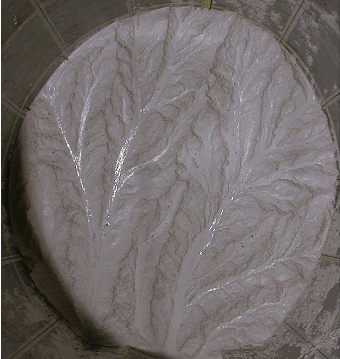
Figure 5-4. Vertical photograph of landform in erosion facility after a steady balance between uplift and erosion has been reached. Width of basin is 87 cm. Maximum relief (from top of image to bottom) is 17.8 cm ( 1 H_r ). Note the narrow valley in the lower center of the basin. Its upstream end is beheaded.
