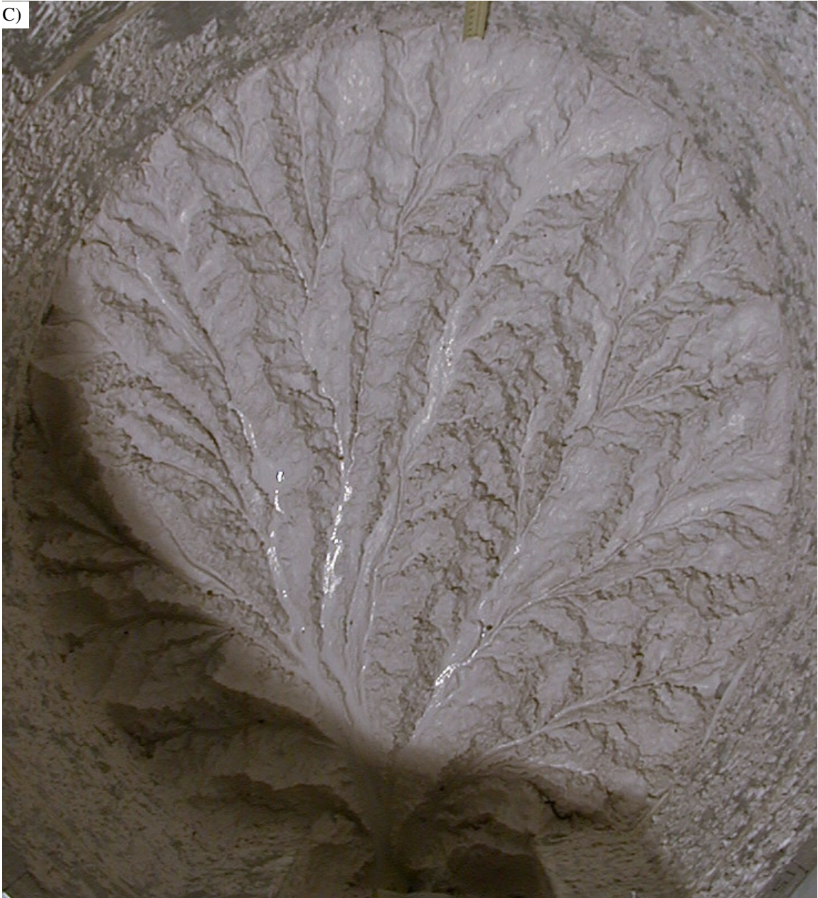
Figure 2-24. C) Surface after additional 18 cm of erosion ( 1 H_r ), run 4. Drainage divides are irregular and crenulated. Many channels appear quite narrow. A long narrow terrace has formed in the lower left center trunk stream. A hillslope failure is visible (smooth 'creamy' area, long left center ridge) that has dammed a channel. Width of the basin is 87 cm.
