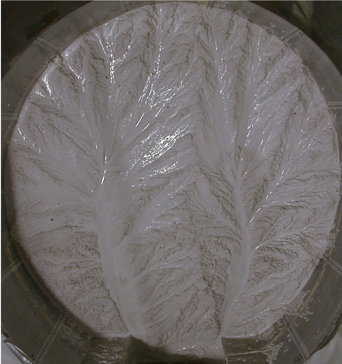
Figure 2-37. Surface after mist apparatus adjustment, run 7 (~3 cm of erosion has occurred). Width of basin is 87 cm. The center ridge has migrated toward the right side of basin, which has roughened considerably. The upper left of the basin has smoothed.
