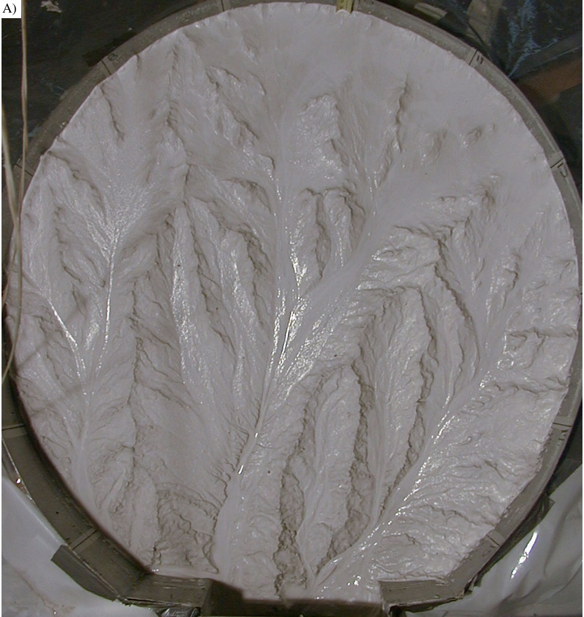
Figure 2-30. A) Surface nearing complete dissection, run 6. Note the remnant plateau at the top of the photograph. Maximum relief is 12.7 cm. Basin width is 87 cm.
