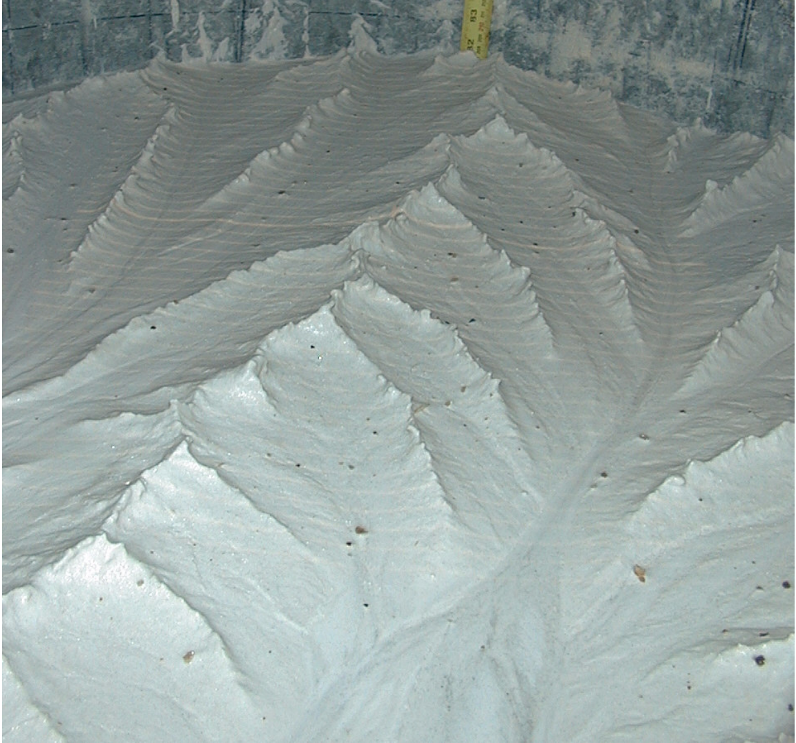
Figure 2-32. Declining relief phase at fixed base level, run 6. Width of image is ~40 cm. Surface is very smooth, with a skeletal ridge network. Local relief is 1-2 cm, and the maximum relief is ~11 cm.
