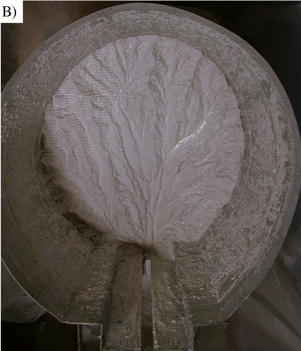
Figure 2-19. Vertical photographs of A) surface at complete dissection; and B) surface at the end of the run, after \sim 3 H_r of erosion. Basin width is 87 cm. Note the poor correspondence of ridge locations between the two images.
