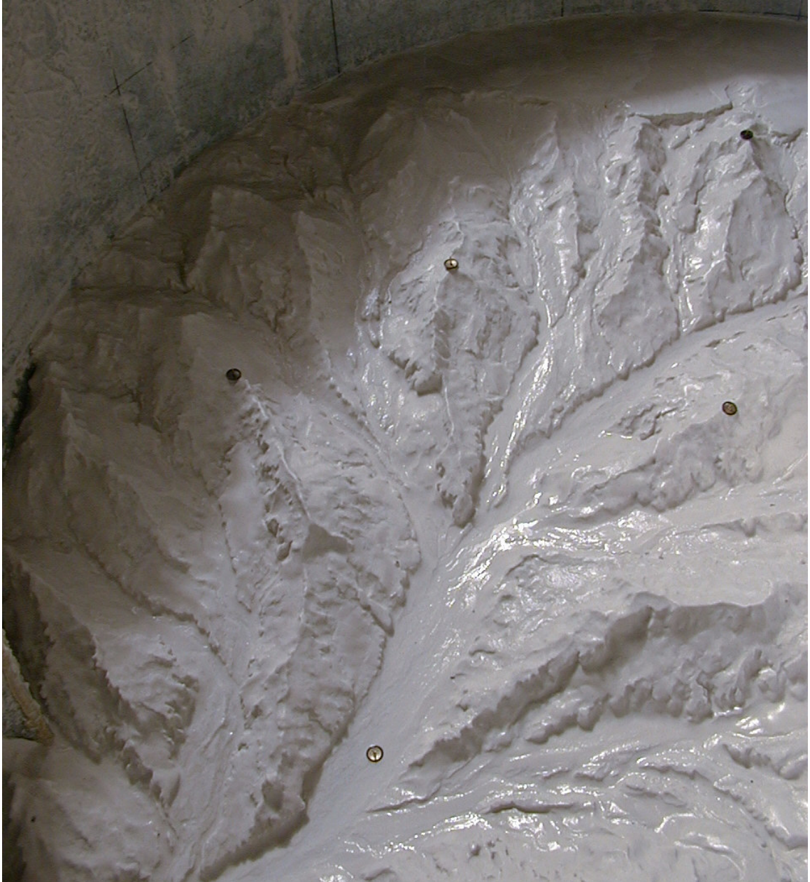
Figure 2-17. Oblique view of surface prior to complete dissection. Width of image is ~40 cm. Slumping is apparent in the lower right of the image. Ridges and valleys are relatively smooth.
