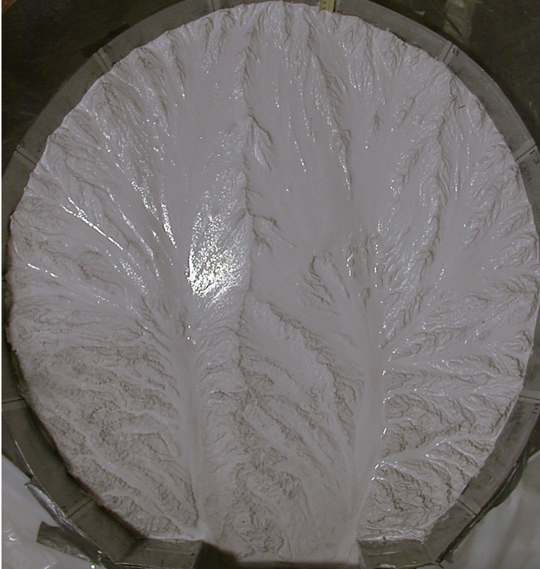
Figure 2-35. Surface at complete dissection, and prior to the adjustment to the mist apparatus at t = 66,000 s. Width of basin is 87 cm. Two main sub-basins have developed. Knickpoints are visible in both main trunks in the center of the basin. Note the smooth character of the surface upstream from the knickpoints. Large spatial variation in rainfall rates exist for this run, with the highest rates ( \sim 100 \mu\text{m/s} ) in the upper center of the basin, and the lowest rates ( \sim 10 \mu\text{m/s} ) occurring near the outlet.
