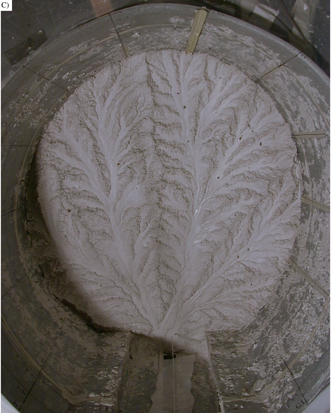
Figure 2-26. C) Surface at the end of the run, run 5. Ridges are rough and crenulated. Maximum relief is 18.3 cm.
