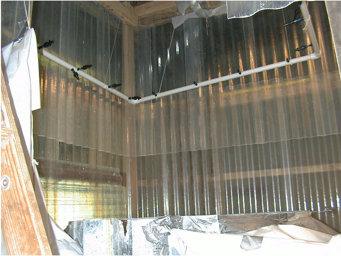
Figure 2-33. Rainfall apparatus arrangement, run 7. Four misters on the left and five on the right side (not in view) of erosion facility generated a higher intensity rainfall. Two different nozzle orifices were used. Changing the orifice size changed both the intensity and spatial distribution of rainfall.
