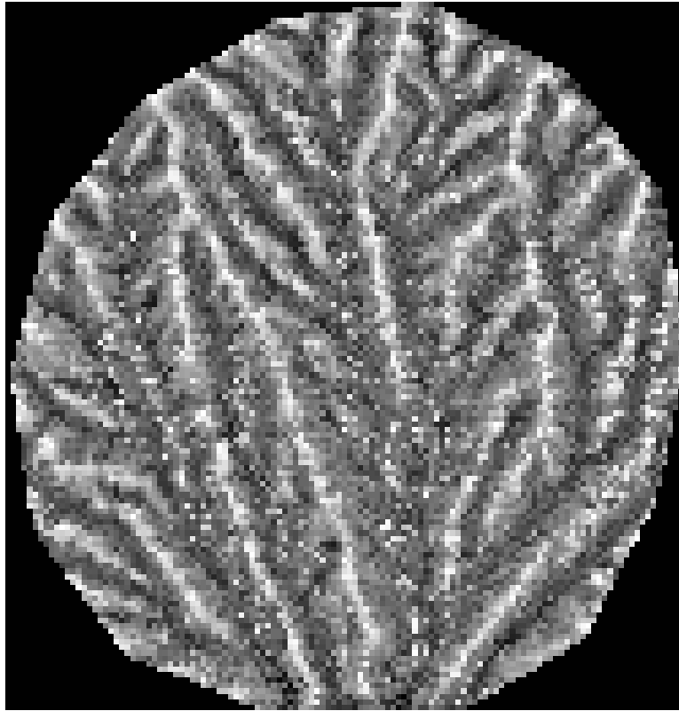
Figure 2-13. Local relative height plotted as a gray-scaled height map. White represents points that are higher than their adjacent neighbors (peaks). Dark values represent locations that are lower than their neighbors (depressions). Moving window size is 7 x 7 pixels (4.9 x 4.9 cm). Local relative height captures the ridge structure of the topographic surface. Valleys are less well defined. Grid spacing is 7 mm, with 12,770 data points in the grid.
