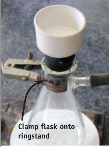
**Step 2:** Clamp the filter flask onto your ringstand so the flask will not tip over. Attach a piece of rubber vacuum tubing.
