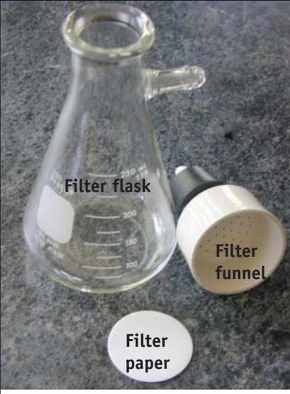
**Step 1:** You need a glass or plastic filter flask (with sidearm), a plastic or porcelain funnel, and a piece of filter paper.
