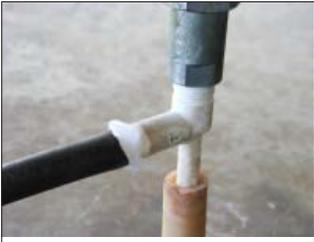
**Step 4:** Plug the vacuum tubing with the plastic fitting onto the water spigot in front of your lab station. Turn on the water all the way and test to see if a vacuum has been created in your flask and funnel.
