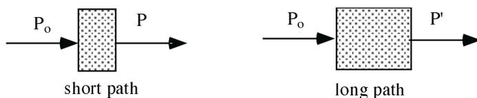
We shine light of the same intensity ( $P_0$ ) on both containers. In the first case the light has to travel through only a short distance, whereas in the second case it has to pass through a much longer length of the sample. We might deduce that in the second case more of the light will be absorbed or cut off, since the path length is longer. In other words, absorbance increases as path-length increases.
