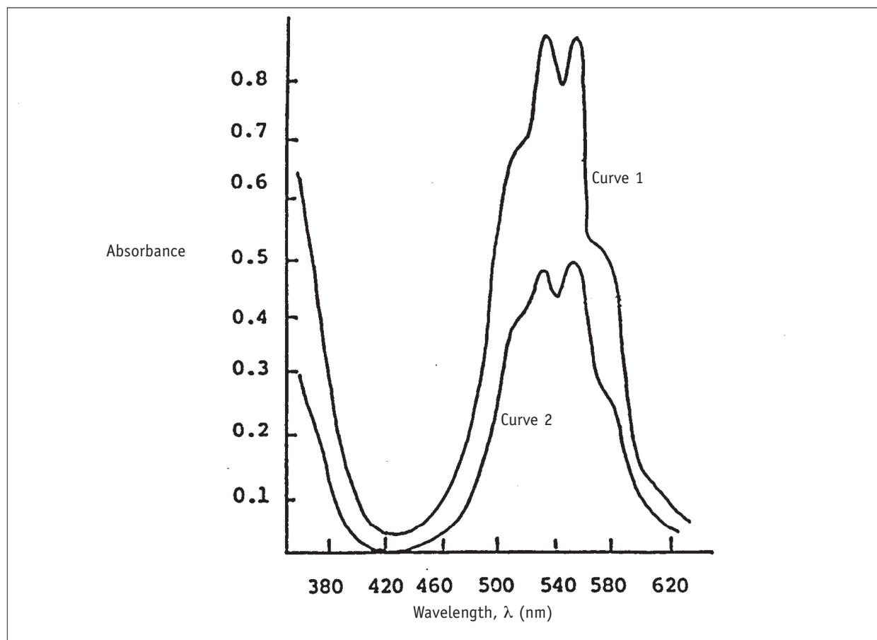
**FIGURE** The absorption spectrum of solutions of potassium permanganate ( $\text{KMnO}_4$ ) at two different concentrations. The solution for curve 1 has a *higher* concentration than that for curve 2.
