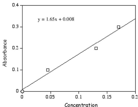
Slope of the best straight line through the data points in the calibration plot is 1.65. Plot intercept is 0.008.
