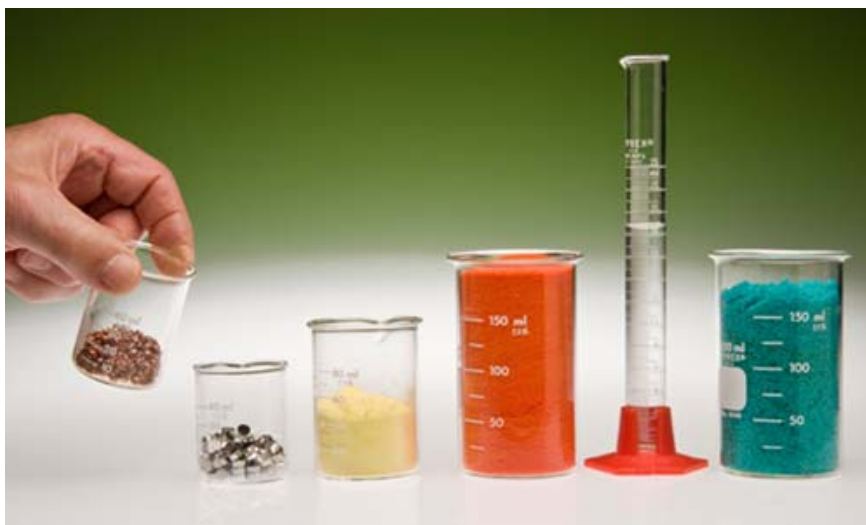
Interactive Figure 3.1.1 Recognize How the Mole Connects Macroscopic and Atomic Scales One mole quantities of (from left to right) the elements copper, aluminum, sulfur, and oxygen and the compounds potassium dichromate, water, and copper(II) chloride dihydrate.
