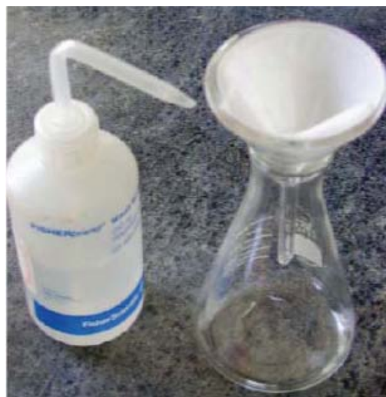
Step 4: Place the filter paper in the funnel. Moisten the paper with a few drops of distilled water from your squeeze bottle.
