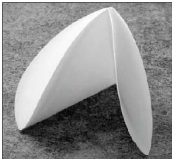
Step 1: Fold the filter paper in half, and then in half again
