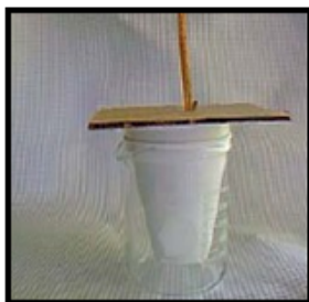
(b) Two cups together, supported by a beaker. Cover in place with a thermometer through the hole in the cover.
