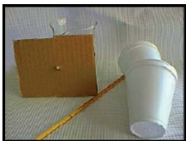
(a) Calorimeter consists of a thermometer, two styrofoam cups, paper cover, and beaker.
