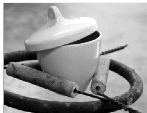
Figure The bottom of the porcelain crucible will glow cherry red when it is heated properly.
