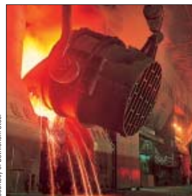
A reaction requiring a higher temperature so that \Delta S_{\text{univ}}^\circ is positive. Iron is obtained in a blast furnace by heating iron ore and coke (carbon). See Exercise 19.5.
