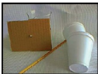
(a) Calorimeter consists of a thermometer, two styrofoam cups, paper cover, and beaker.
