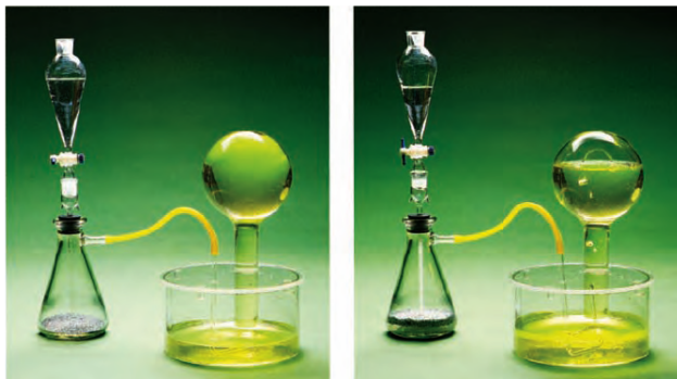
Figure 10.X. Collecting a gas by water displacement
