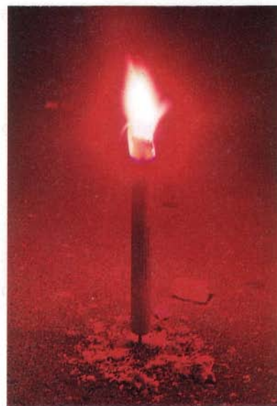
Figure 4-6 A red signal flare. The red color arises from light emitted by electronically excited strontium atoms.
