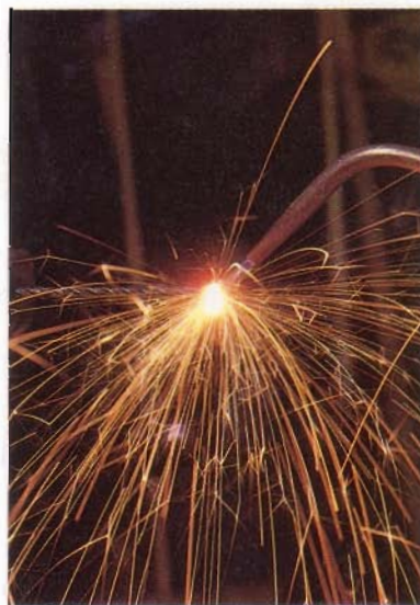
An oxy-hydrogen torch. The flame temperature is about 2500°C.
