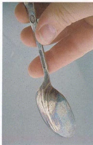
Silver sulfide is a black, insoluble solid that appears as a dark tarnish on the surface of silver.
