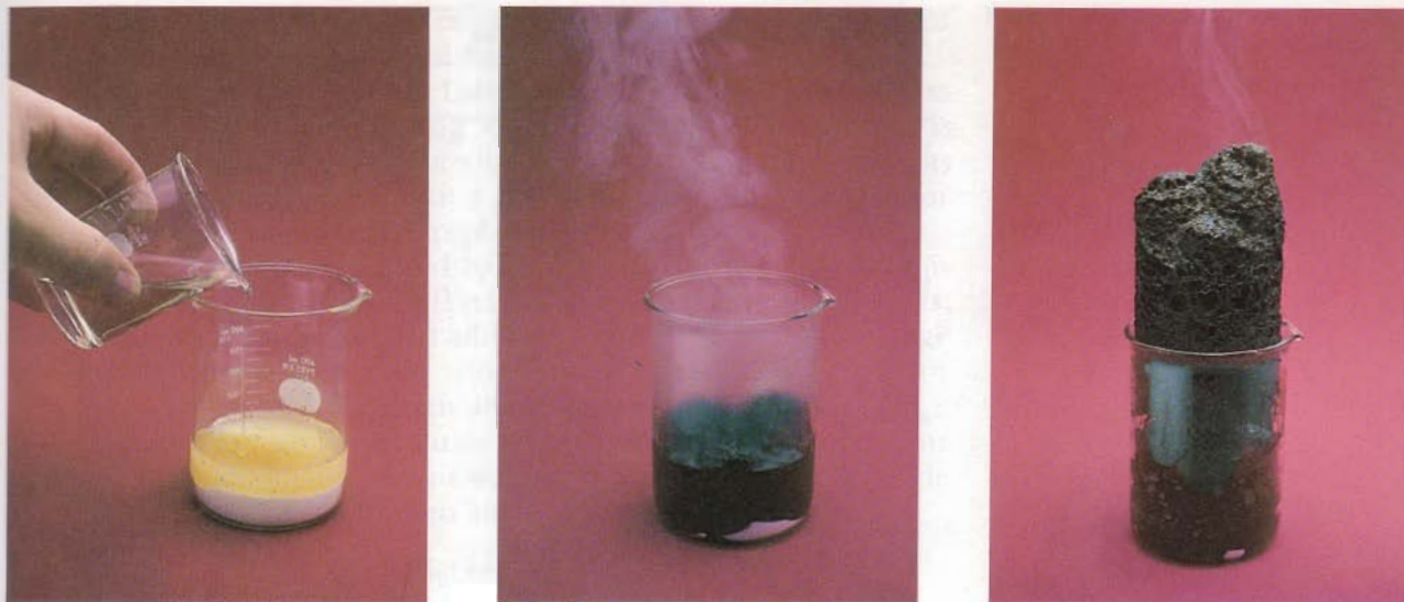
Figure 8-8 Concentrated (98%) sulfuric acid is a powerful dehydrating agent capable of converting sucrose to carbon.
