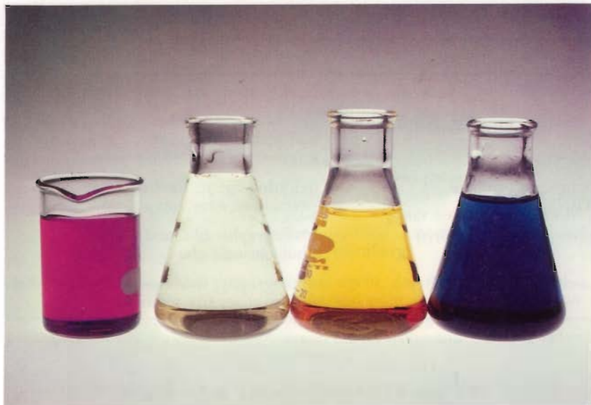
Figure 9-4 Various solutions of iodine. Left, I_2 dissolved in CCl_4 . Center left, I_2 dissolved in KI(aq) . Center right, I_2 dissolved with water. Right, I_2 dissolved in KI(aq) with starch added to the solution.
