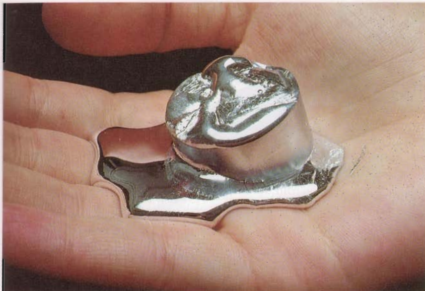
Figure 5-6 Gallium metal has a melting point of 30^{\circ}\text{C} , so a piece of gallium melts when held in the hand (human body temperature is 37^{\circ}\text{C} ). Only two elements are liquids at room temperature ( 20^{\circ}\text{C} ). One is the metal mercury, and the other is the nonmetal bromine.
