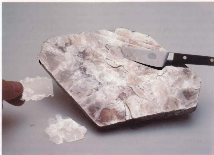
Figure 6-14 The ease with which the mineral mica can be separated into thin sheets is a direct consequence of the existence of polymeric silicate sheets with the composition (\text{Si}_2\text{O}_5^{2-})_n .
