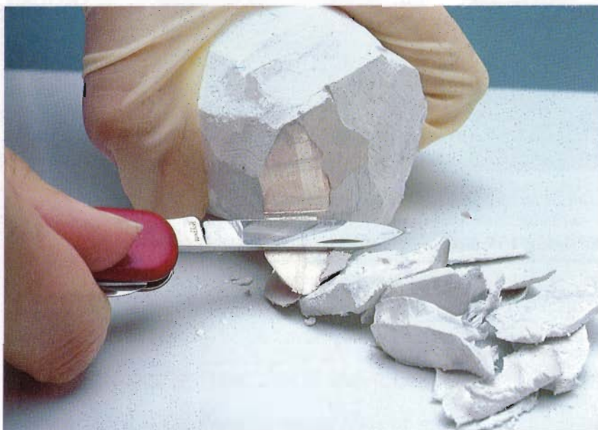
Figure 3-2 The Group 1 metals are soft. Here we see sodium being cut with a knife. Note the shiny surface of the freshly cut metal and the tarnished surface that results on exposure to air.
