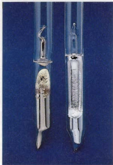
Cesium (which is a gold color) and rubidium (silver). They are stored in vacuum tubes to prevent them from reacting with the air.
