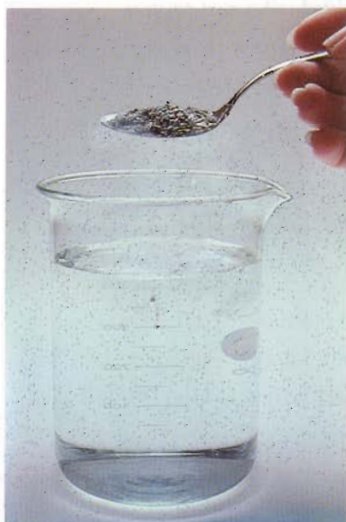
Calcium hydride (CaH 2 ), a white crystalline ionic solid, reacts readily with water to produce hydrogen gas.
