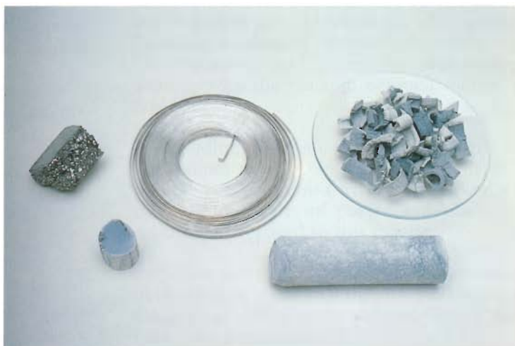
The Group 2 elements. Top row; beryllium, magnesium, and calcium. Bottom row; strontium and barium.
