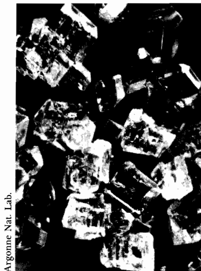
Figure 10-2 Xenon tetrafluoride crystals. Xenon tetrafluoride was first prepared in 1962 by the direct combination of \text{Xe}(g) and \text{F}_2(g) at 6 atm and 400^\circ\text{C} .
